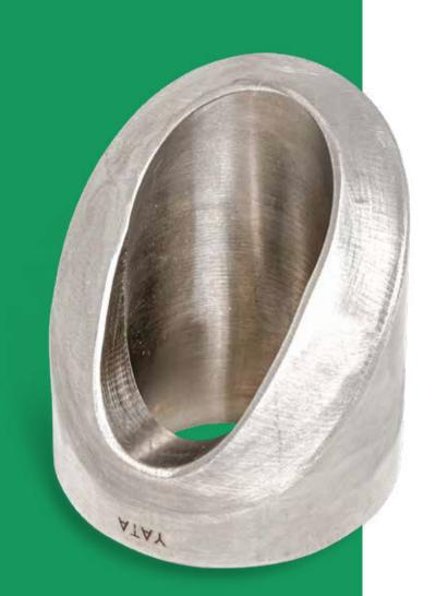
ElboMegalets are Branch outlets used to connect a pipe to an elbow or a bent pipe. ElboMegalets connections are in all sizes, types, bores, and classes, in a wide range of stainless steel, chrome-moly, and other alloys. The branch ends can be butt-welded (BW), socket-welded (SW), or threaded (usually NPT). ElboMegalets meet the reinforcement requirement of applicable piping codes i.e., ASME B31.1, B31.3, B31.4, and B31.8.
