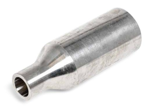
Eccentric Swage Nipples are fittings used to connect pipes of different sizes. Eccentric Swage Nipples are manufactured in accordance with the applicable Standard Practice MSS-SP-95 and can be supplied with bevel, plain or threaded ends.
