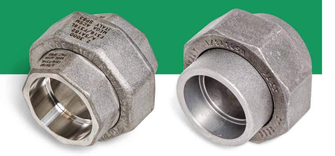
Unions are three-piece fittings used for mobile connections of piping. Obtained from forgings, Unions are available in all sizes up to 4in, classes 3000 and 6000, in a wide range of carbon steel, stainless, chrome-moly, and other alloys. The ends can be socket-welded (SW), threaded (usually NPT), or butt-welded (BW). Unions are manufactured in accordance with the applicable Standard Practice MSS-SP-83 or BS 3799.
