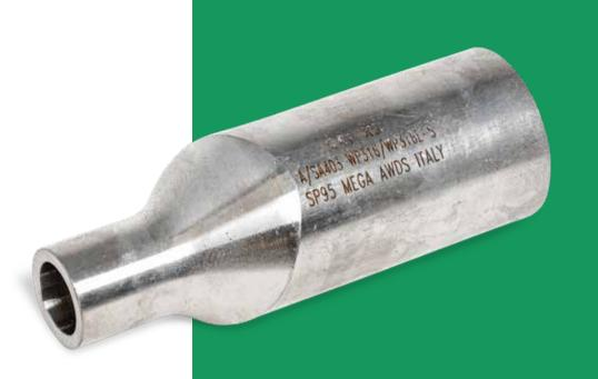
Swage Nipples are fittings used to connect pipes of different sizes. Swage Nipples are manufactured in accordance with the applicable Standard Practice MSS-SP-95 and can be supplied with bevel, plain or threaded ends.
